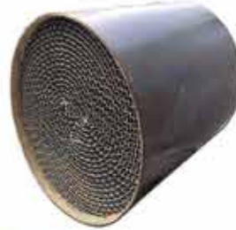
90603204 Diameter= 108mm Length= 100mm 100cpsi(Cells) PE (Perforated Foil to reduce weight & Backpressure)
