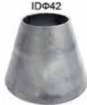
ID \Phi 42 \Phi 80 C-80 Height = 50mm SUS304
