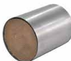
SUB62 Diameter= 120mm Length= 130mm Euro6 / 200cps(Cells) High Loading / Premium Quality
