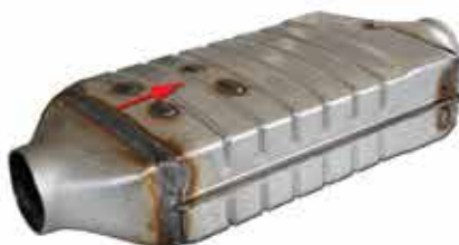
90631130 Body Diameter= 175x80mm Total length= 405mm Inlet-Outlet= OD60 DPF Oval / Metallic
